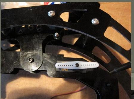
Step 21: Install Roll servo and attach linkage Roll servo linkage (provided in newer kits) You may need to try different servo horns to find the right one that gives you the most roll. (Make sure linkages are tight and have no movement. Most servo problems comes from unsecure and loose connections.)
