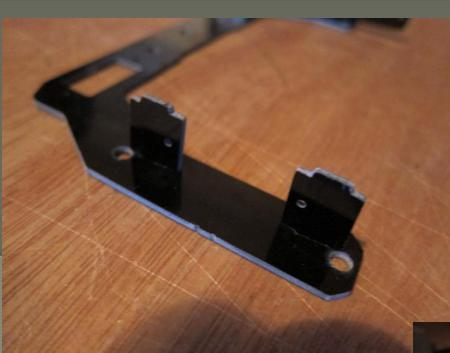
Step 16: Insert Servo Mount tabs into camera frame. (trim as needed for a perfect fit)
