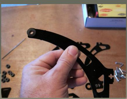
Step 3: Insert Rubber Grommet into leg assembly – Do this for each of the 4 legs
