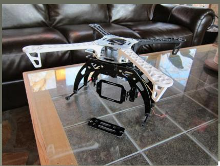
Final NAZA Flame Gear Standard Mount installed on F450 (GoPro and 450 not included)
