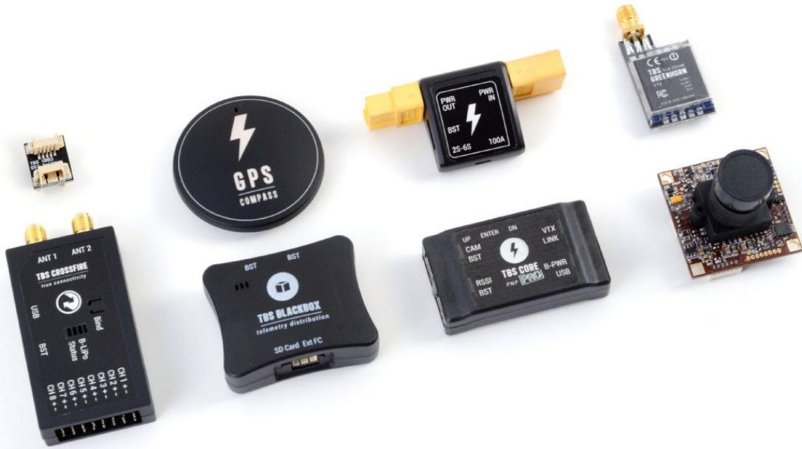
The compact receiver unit fits everything from small multirotors to very large airplanes. The receiver is capable up to 8.4V and needs at least 4.5V input voltage. This can be applied to any of the eight servo headers, e.g. a servo cable from a ESC with BEC, or a stand-alone BEC, with a suitable amperage rating - min. 1A recommended. Make sure that adequate power is available by letting the model run for a few minutes with servos connected, and check your BEC temperature.
