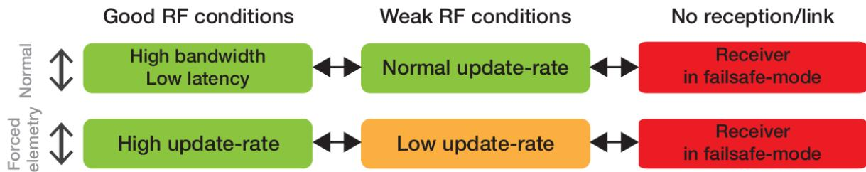
The link has two operation modes which are based on three RF profiles. Every mode has its pros and cons. TBS CROSSFIRE always switches between two RF profiles, depending on the current link health while you are flying. The two profiles used is according to your decision to use "Normal" or "Force telemetry" modes. Which two RF profiles are in use for each mode is showed in the diagram above. We recommend to use the default "Normal" mode as it fits the most of the use cases.
