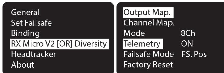
For the CROSSFIRE DIVERSITY RX, change “Output 7” to “CRSF RX” and “Output 8” to “CRSF TX”. While on the CROSSFIRE MICRO V2 RX, change “Output 1” to “CRSF TX” and “Output 2” to “CRSF RX”.
