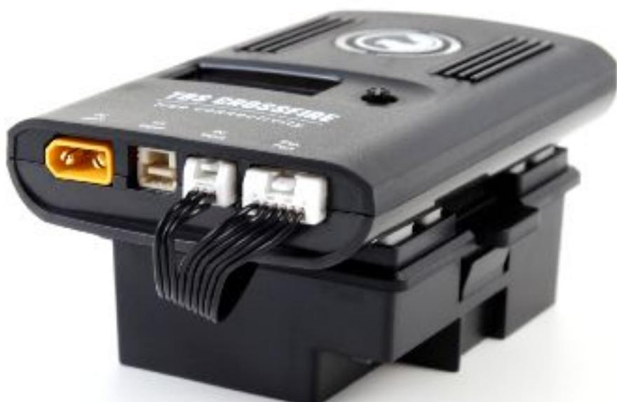
Insert the JR-adapter into the slot on the back of the radio, remove the adhesive sheet from the TBS CROSSFIRE back and align the four studs with the matching holes on the transmitter. Connect the 3-pin to the left port (RC) and 6-pin cable (expansion) to the right port on the transmitter.
