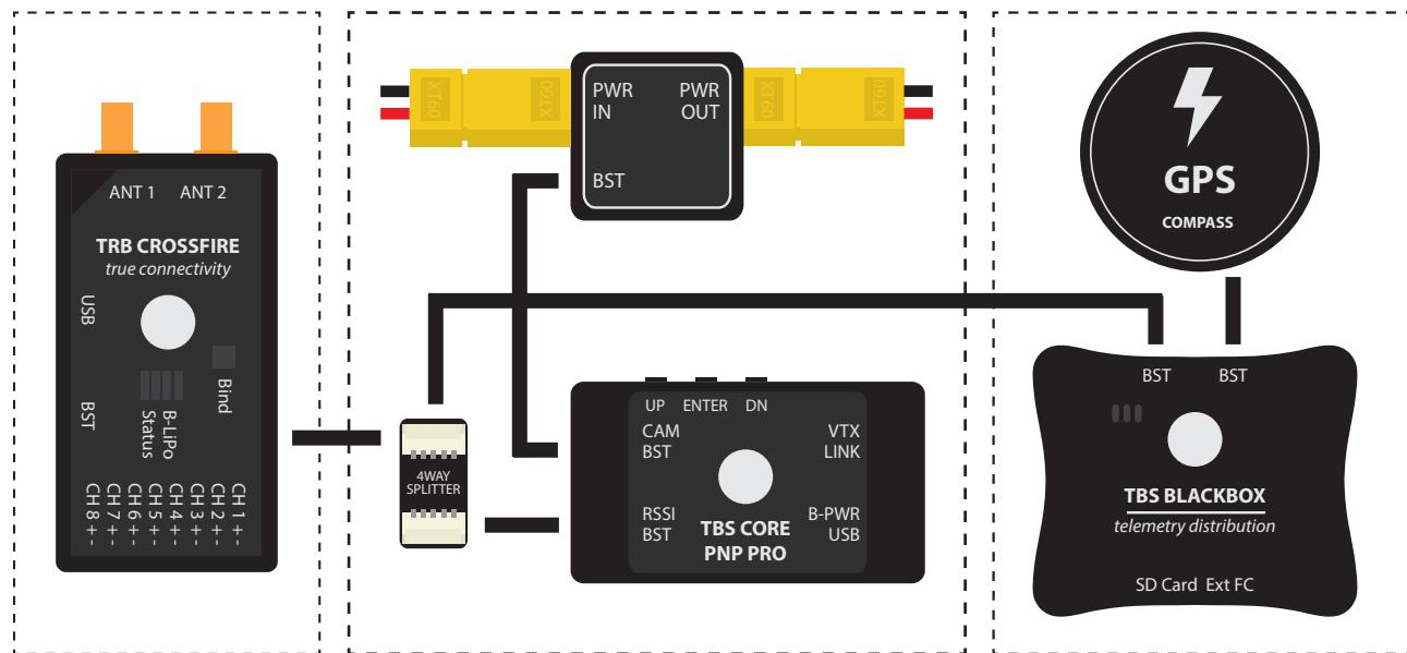
Flight Controller provides 5V via ESC/BEC to all devices
