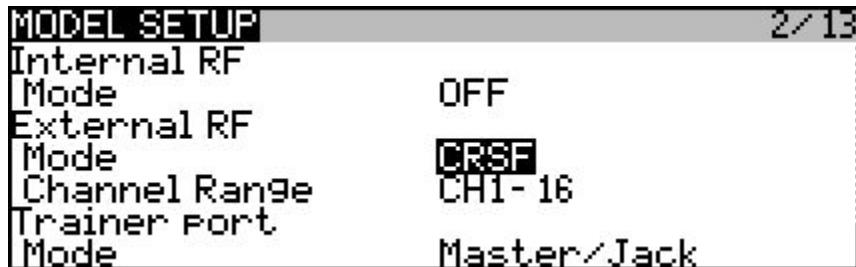
On the CROSSFIRE transmitter OLED display, you should now see “RC Input: CRSF”, meaning you have CRSF enabled and running.
