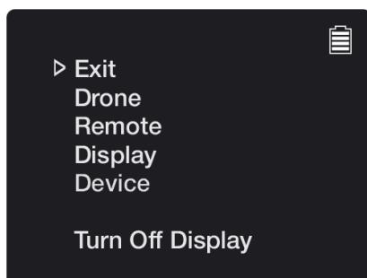
Enter the configuration menu by holding the jog-scroller for 3 seconds
