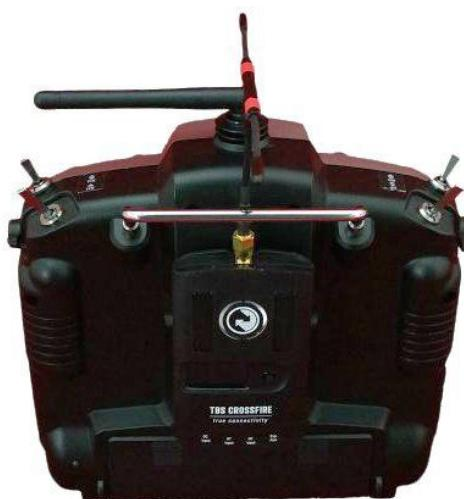
Correct transmitter antenna mounting direction
