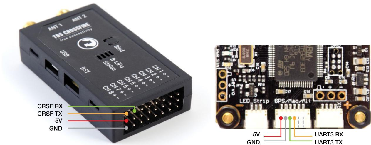
In addition to the CRSF serial connection, you might want to connect BST (BlackSheep Telemetry) between the CROSSFIRE RX and COLIBRI to provide more telemetry and make changes remotely on the CORE PRO (if connected) or FPVision (if part of the POWERCUBE).
