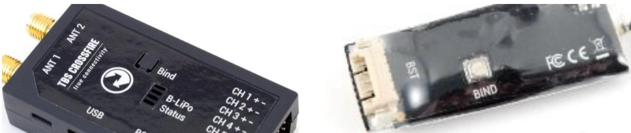
Within a few seconds the process will finish with a "Binding complete" message. The receiver has now stored the unique serial number of that particular CROSSFIRE transmitter. If it doesn't bind, please verify that your firmware is to the newest version on both the receiver and the transmitter.
