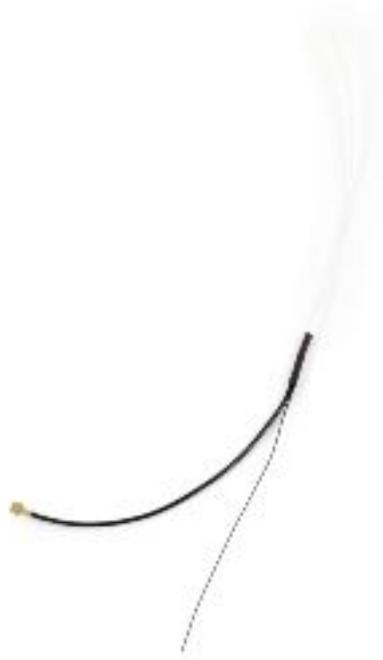
Micro receiver antenna with U.FL connector
