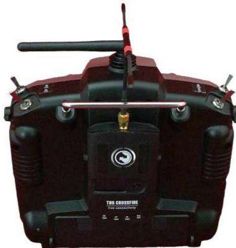
Correct transmitter antenna mounting direction
