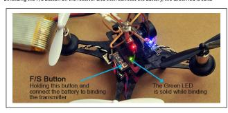
3.Go to the Receiver [Bind] option, and ENT to Bind with the receiver, The transmitter beeps
