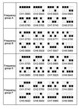
Move Dip 1/2/3/4/5 to change the channel, Move Dip 6 to reverse the display
