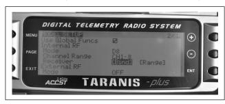
4. The green LED on the receiver will turning off, this indicates that the bind process was successful Reconnect the battery for the QX90, and the green LED on the receiver is solid again.
