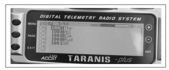
$2. The\ QX90\ BNF\ was\ set\ AUX1(CH5)\ to\ ARM/DISARM\ the\ motor\ before\ shipping,\ you\ can\ also$ customize it
