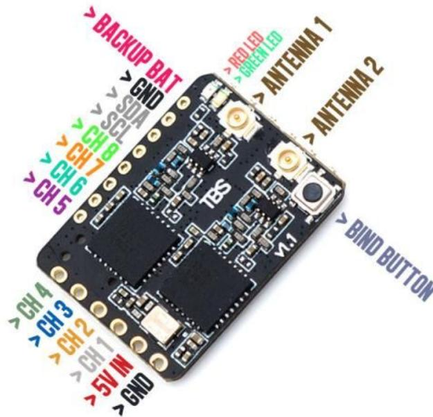
Connect the antenna with the U.FL connector to the socket on the receiver. To ensure that it does not disconnect or unseat, run the coax cable across the receiver board over to the servo channel end and secure it with the heat shrink-tubing.
